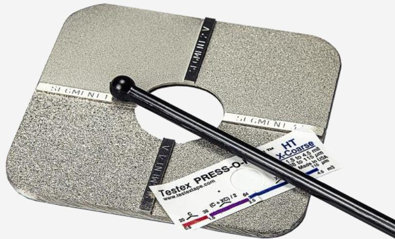
Remove a single piece of Replica Tape from its release paper. The replica material is the square, white plastic film in the centre. A bulls eye circle of paper should remain behind on the release paper (this is not used in the measurement).
