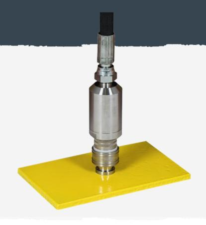
Check that no adhesive has been left in the dolly hole by trial fitting the Dolly Plug.
