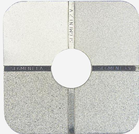
When steel has been blast-cleaned, the surface consists of random irregularities with peaks and valleys that are not easily characterised. Because of this random nature, experts have recommended that the profile should be identified as either angular (where grit abrasives have been used) or dimpled (where shot abrasives have been used) and that they should be graded as fine, medium or coarse with each grade being defined by limits specified in ISO 8503.
