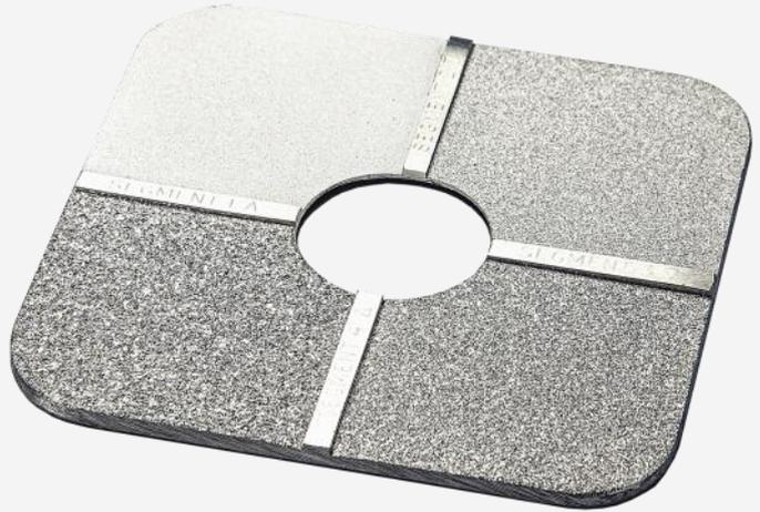
Place the selected Comparator against an area of the test surface. Compare in turn the test surface with the four segments of the Comparator, using the Illuminated Magnifier if necessary. If the Illuminated Magnifier is used, place it so that the test surface is viewed simultaneously with a segment of the Comparator.
