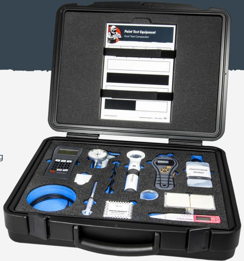
Testex Tape / Testex Gauge. Surface Profile measurement of blast-cleaned steel.
