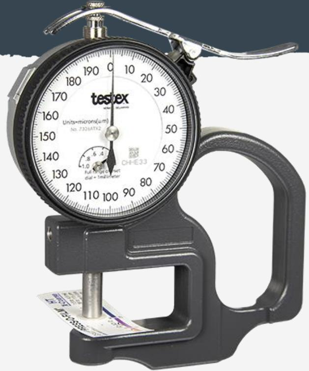
The Testex Gauge is used to measure the Testex Tape replica and determine the average maximum peak-to-valley height of the blasted profile.
