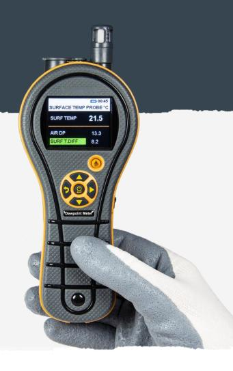
The steel surface temperature generally should be at least 3°C above the dew point when paints are applied. Below this temperature the Dewpoint Meter will sound an alarm and the display colour will change to warn you that the surface conditions are not suitable too paint.
