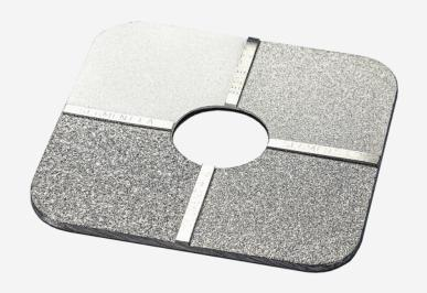
Place the selected Comparator against an area of the test surface. Compare in turn the test surface with the four segments of the Comparator.
