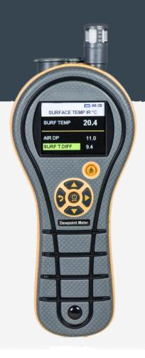
Remove the rubber cap from the infra red sensor and point at the substrate. Press the infra red temperature button (IRT) and the measurements will show on the display.
