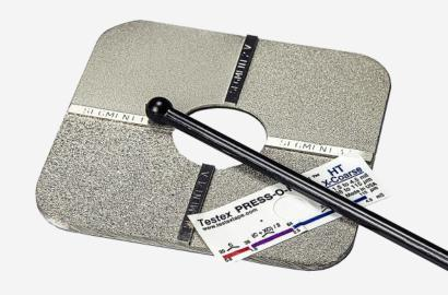
Remove a single piece of Testex Tape from its release paper. The replica material is the square, white plastic film in the centre. A bulls eye circle of paper should remain behind on the release paper (this is not used in the measurement).
